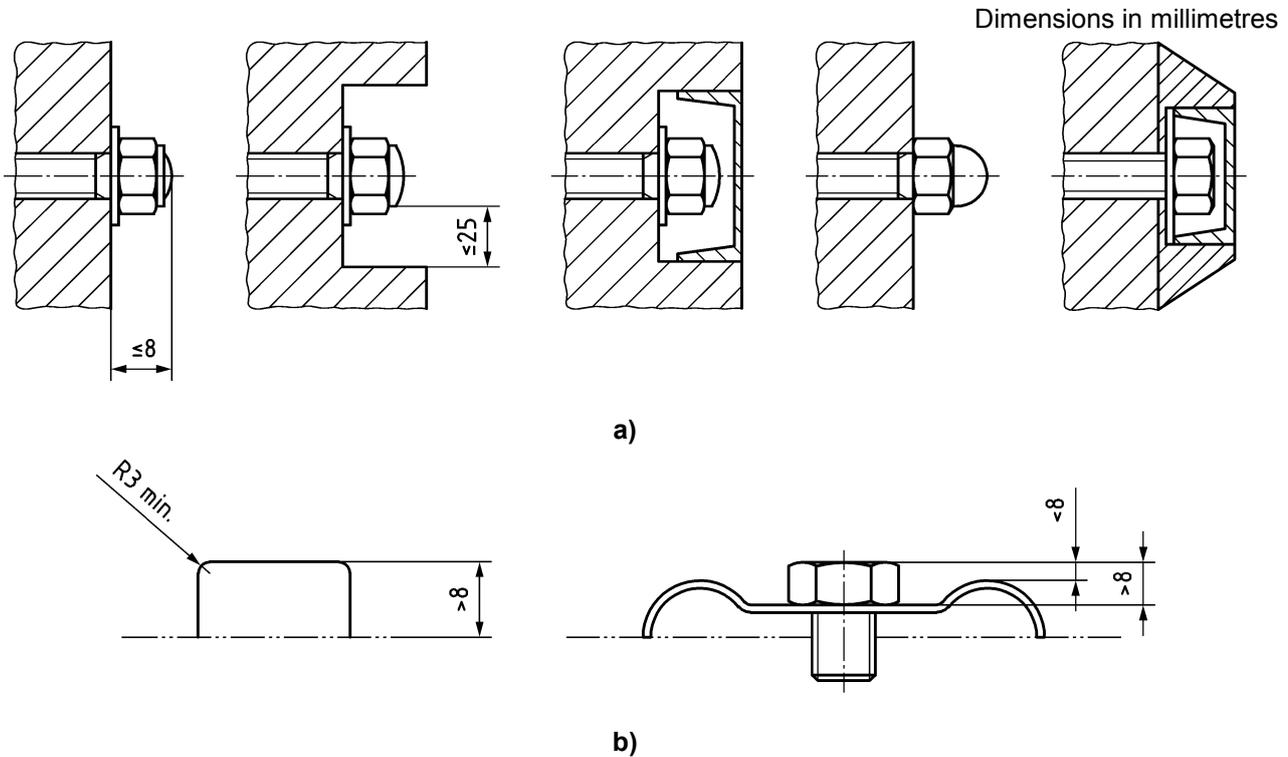
Figure 6 — Examples of protection and permissible protruding parts
