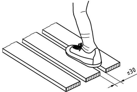
**Figure 8 — Measurement of gaps limited to 30 mm**
