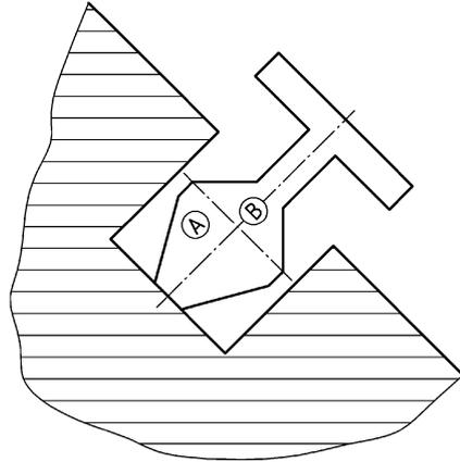
a) Pass if front section fully enters opening to a maximum depth of 265 mm (template shoulder depth)
