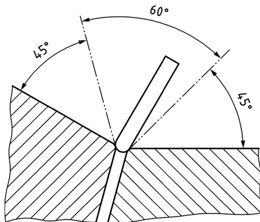
**Figure 21 — Movement of the 8 mm diameter finger probe**
